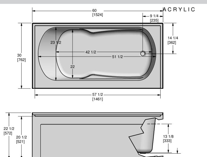
Measurement tolerances ± 1/4" (6.3mm)
